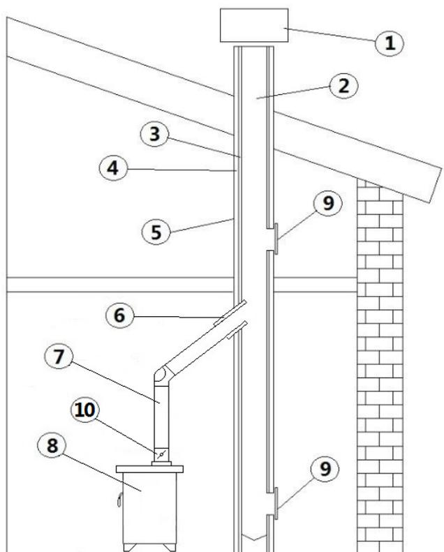
Fig. 4 - Chimney components
