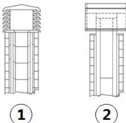
Fig. 3 - Anti-wind chimney pots
